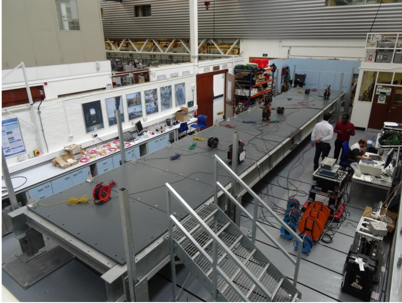
Figure 4. The reconfigurable steel footbridge located at the laboratory of the Vibration Engineering Section of the University of Exeter.
