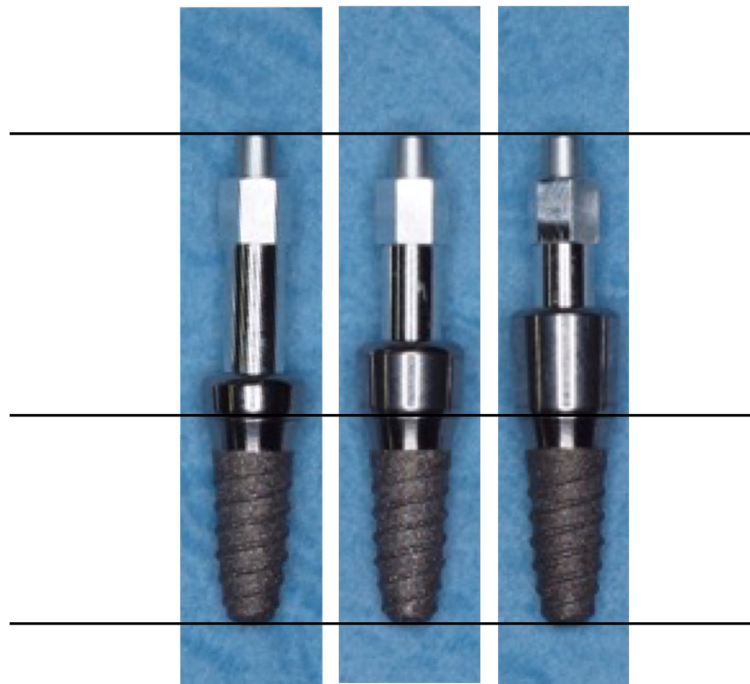
Figure 5. Healing plugs of different heights (2/3.5/5 mm) placed on the implant; it can be seen that the total height of the SmartPeg is the same (distance to the bone/implant shoulder) so as not to distort the resonance frequency analysis (RFA).
