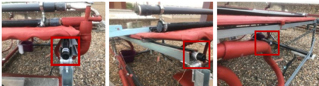
Figure 7. In situ relative humidity measurements
