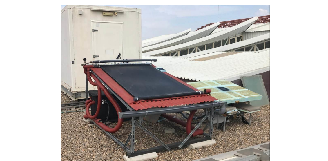
Figure 11. Type 1 test: assessing mean nocturnal dissipation power in operating mode 1
