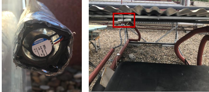
Figure 6. In situ measurement of outdoor air temperature
