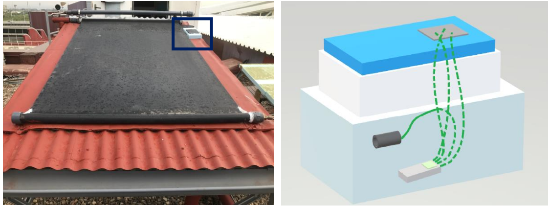
Figure 4. Equilibrium temperature measurement
