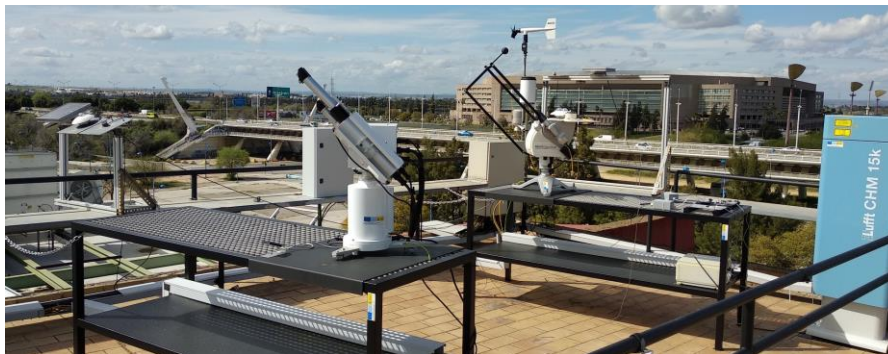
Figure 5. Meteo station and sky meter [48]
