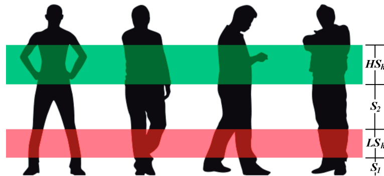
Figure 4. Example of height range segmentation for people detection. In red, the Lower Section; in green, the Higher Section.
