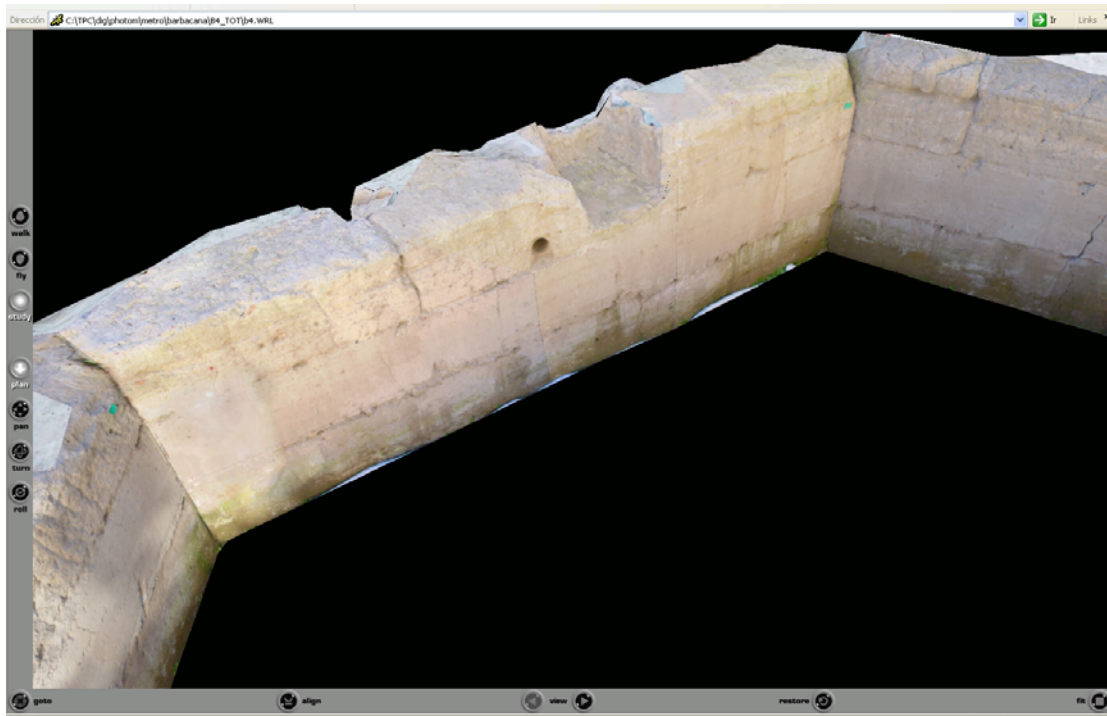
Figure 2. Interactive visualization on the Internet of a fragment of the barbican in VRML format.
