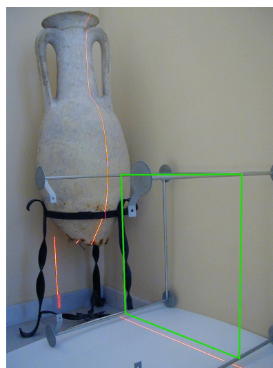
Figure 5: Section produced by the laser plane on the object and the reference profile.
