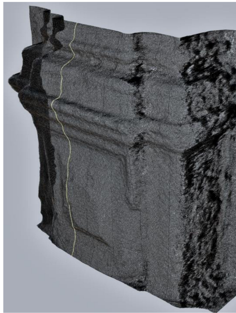
Figure 12. Mesh of the pilaster and the profile created from sectioning using \mathcal{D} plane.
