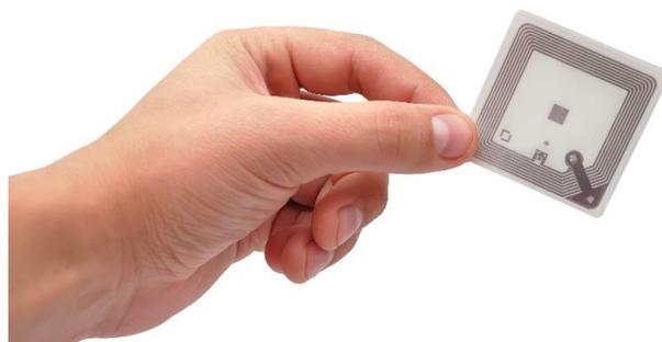
Figura 4.1. Etiqueta RFID. [Fuente: (Witte printed technology, s.f.)]
