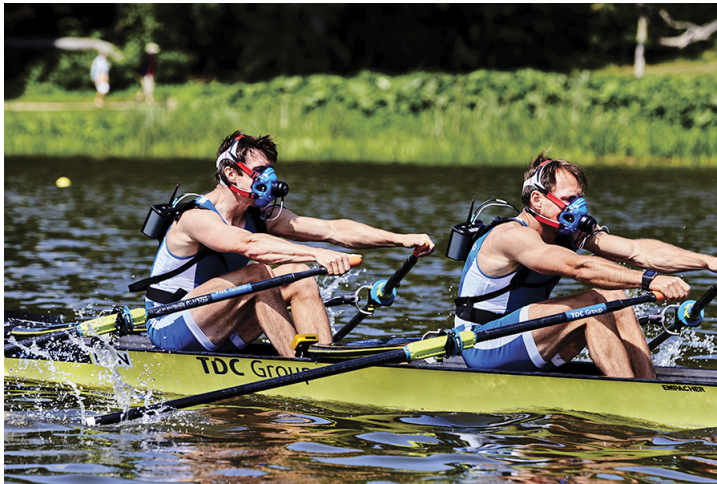
Fig. 3. Cosmed K5 portable indirect calorimeter from http://www.cosmed.com/en/products/cardio-pulmonary-exercise-testing/k5 .
