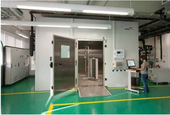
Fig. 2. Direct calorimeter chamber from http://www.directindustry.com/prod/ineltec-france/product-123381-1399577.html
