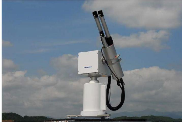
Figura 3-13. Sky Radiometer Prede Pom-02
