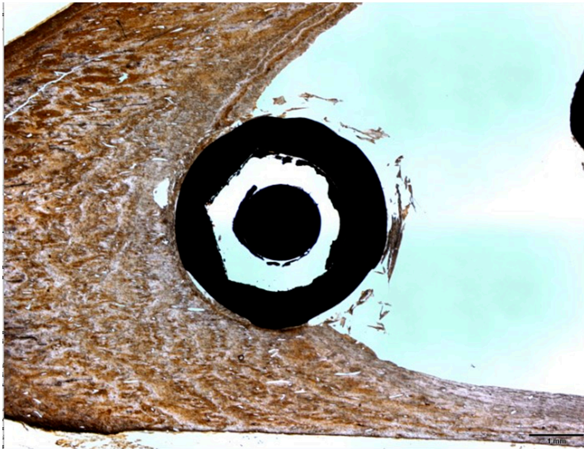
Figure 19. Histological image showing mineralized bone around the HA + AW implant. Von Kossa stain, 5× magnification. The difference in the quantity of the surrounding bone (between left and right sides) is due to the location of the implant in the most distal zone of the tibial metaphysis where bone is thinner. This is an anatomical limitation because this bone has different thickness over its whole length, being thicker on the proximal zone. This image is from a distal zone of implantation. To minimize this effect in all groups, implant locations in the proximal, middle, or distal zones was alternating for reducing this possible limitation/bias.
