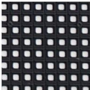
Figura 21. Detalle tecnología SDM (Surface-Mounted Device) [16]
