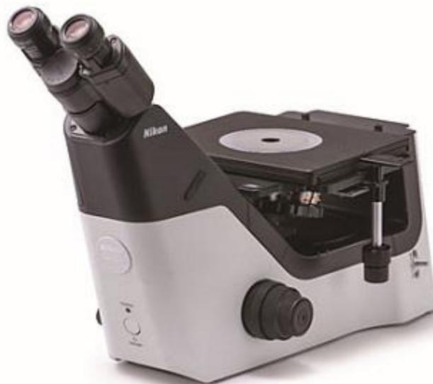
**Figura 53:** Microscopio Nikon Eclipse MA100N
