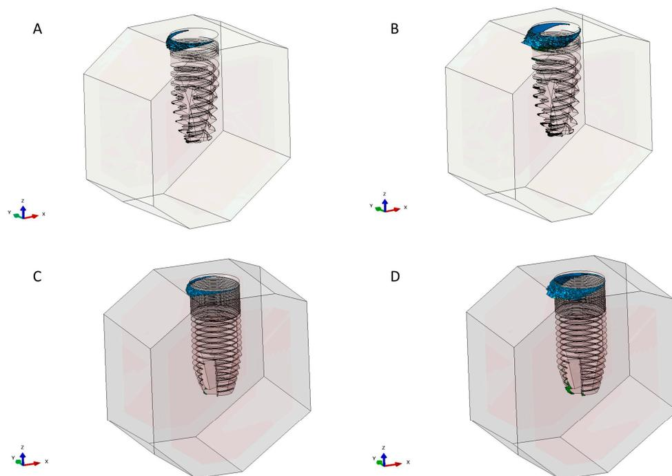
**Figure 5.** Progress of the contact surface loss between the cortical bone and the implant surface over the 10-year period. Bone loss at 5 and 10 years for the M-12 implant (A,B) and Astra implant (C,D).
