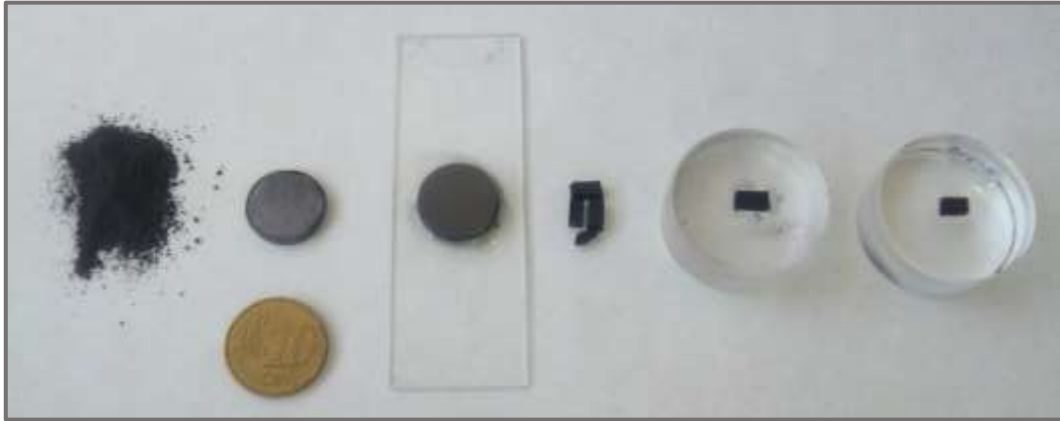
Fig. 2. Samples along the steps of the RCEP preparation protocol. From left to right: CNT-alumina powder after milling and sieving, sintered disc-shaped sample covered with graphite protective wrapping layers for SPS, rectified sample on glass sample holder, rectangular prism sample cuts, embedded sample prism in transparent thermoplastic acrylic mounting material, and polished sample ready to indentation tests. A 0.10 € coin has been used for size reference.
