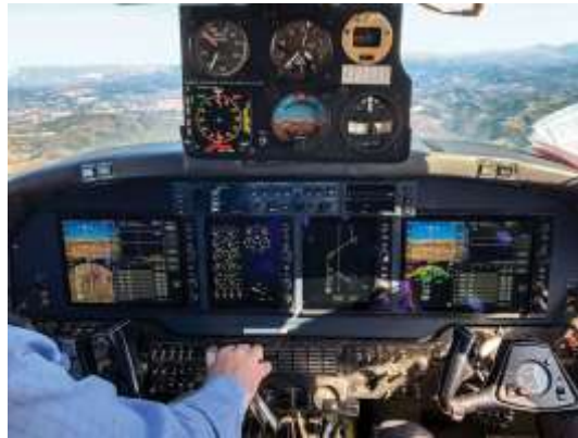
Figure 4-1. Example of avionics systems located at the cockpit. (29)
