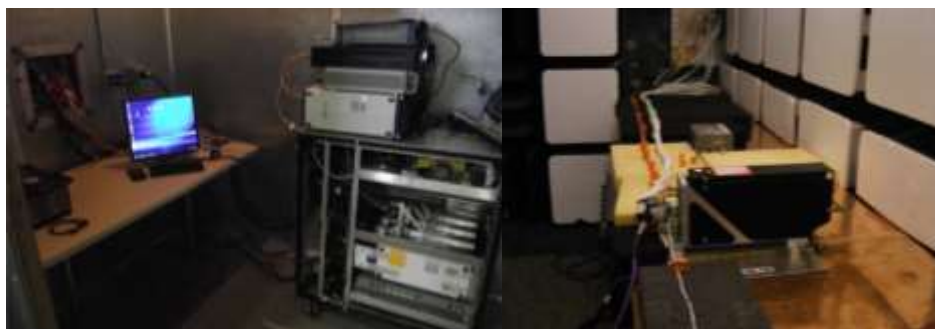
Figure 4-27. Flight Test Pallet outside the EMI Chamber and cable layout. (60)
