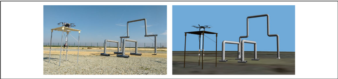
Figure 13. Experiments for aerial manipulation in a mockup scenario emulating pipes in a plant. Real and simulated environments are depicted.
