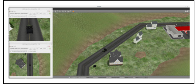
Figure 11. Simulated mockup scenario for MULTIDRONE where two UAVs follow a car taking different types of shots. Views from the two onboard cameras can be seen. UAV: unmanned aerial vehicle.
