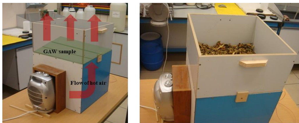
Figure 5. Drying of GAW sample in ETSI laboratory. Details of custom system developed for this work.
