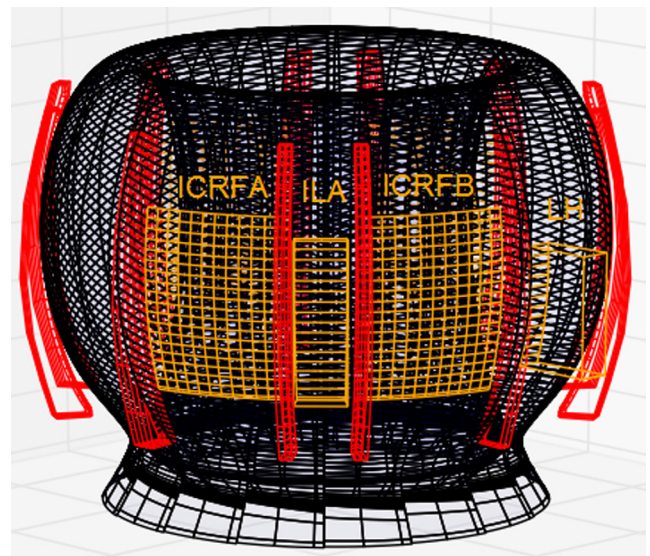
Figure 5. 3D structure of the computational grid, the limiters and the antennas.
