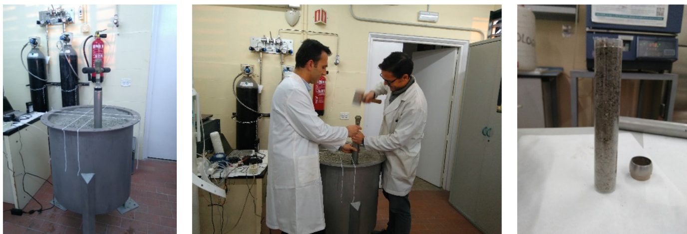
Fig. 2. Sampling material (core) from the reaction chamber after 5 months.
