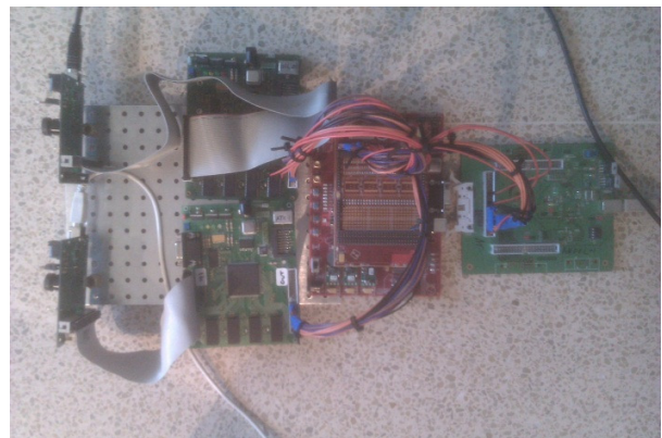
Whole system with two DVS128 retinas (left), two USB-AER boards (middle-left), a Virtex-5 PFGA (middle-right) and the USBminiAER2 (right)
