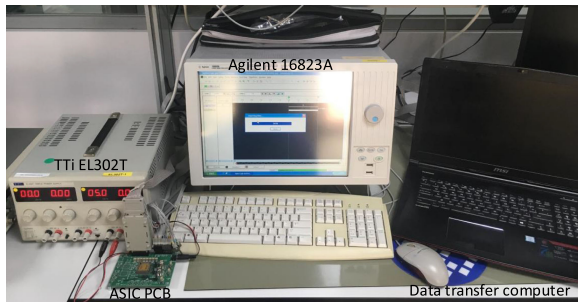
Fig. 9. Laboratory functional test setup, showing the logic analyzer, power supply and the laptop used to transfer data files.
