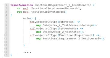
Fig. 12. QVT code of transformation FunctionalRequirement2TestScenario.
