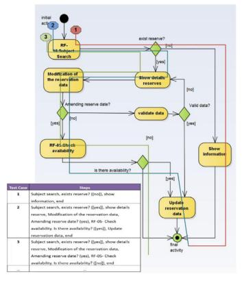
Fig. 2. Example of Round-Trip test pattern.
