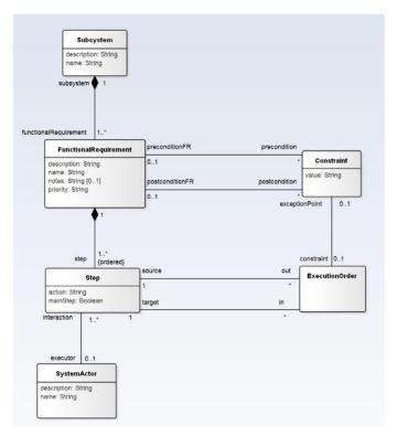
Fig. 5. Functional requirements metamodel.
