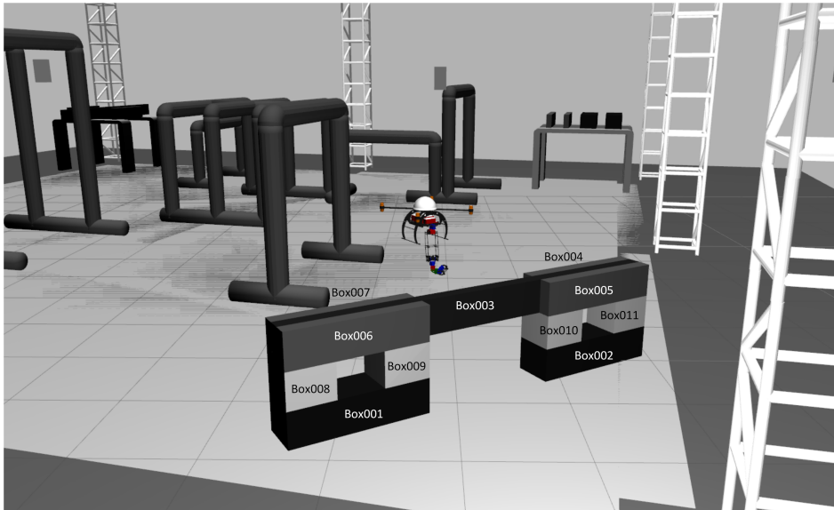
Figure 4.7 Assembly structure for the mission. The structure is composed of eleven parts, enumerated from Box001 to Box011 . All the parts are supposed to have a flat handle from which the robotic arms of the UAVs can pick them.
