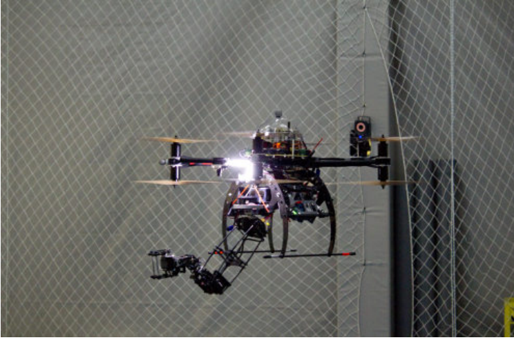
Figure 4.9 Aerial robot prototype equipped with a robotic arm in the indoor testbed located in the FADA-CATEC facilities in Seville (Spain). The model of this prototype has been used in the simulations of the missions.
