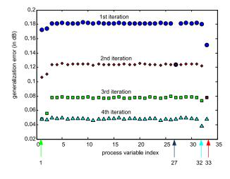
Fig. 5. Generalization error for stepwise addition of process parameters, starting from the DC signatures with supply stress.
