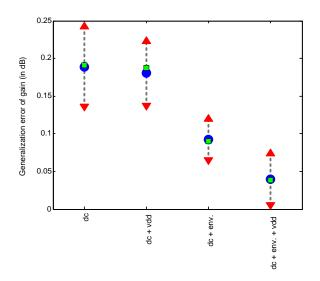
Fig. 2. Generalization error on the prediction of the LNA gain, for four different training scenarios
