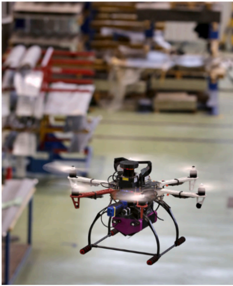
Fig. 1. Aerial robot performing autonomous light object delivery in the Centro Bahía de Cádiz (CBC) Airbus D&S factory.
