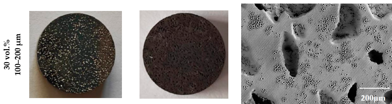
Figure 1. Optical and SEM images of some of the samples studied, before and after FS. All optical images are on the same scale, 3:1 (mm). FD: fully dense sample; 30 vol. %: sample with 30% porosity volume.
