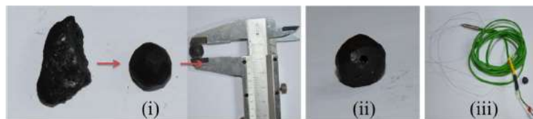
Fig. 3. Processes for the production of experimental coal particle, (i) spherical particles with a certain diameter, (ii) drilled a hole to the particle center, (iii) cemented a fine thermocouple into this hole.
