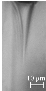
Figure 15. 5 cSt silicone oil meniscus formed in an experiment with Q_1 = 0.05 \mu\text{l h}^{-1} and Q_2 = 10 \text{ ml h}^{-1} .
