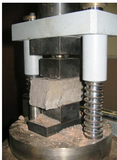
Fig. 1. Specimen under compression test.
