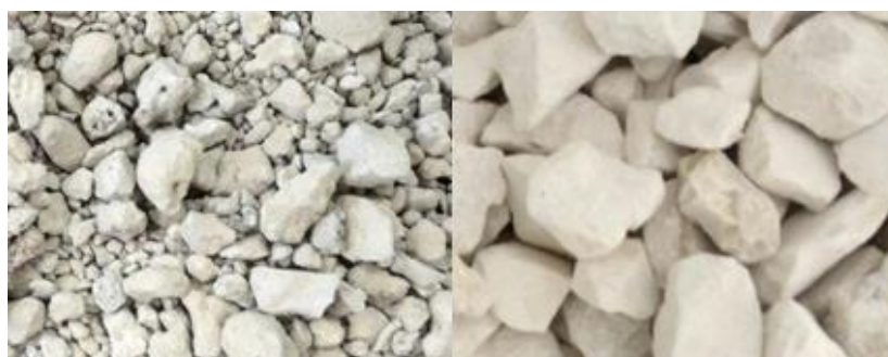
Figure 2. Coarse slag aggregate (left). Coarse natural aggregate (right)
