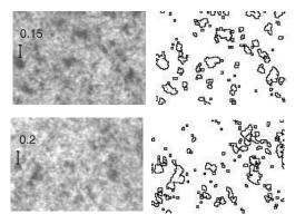
Fig. 5 – Pictures of the aggregates corresponding to different solid volume fractions (size of the bar 150  $\mu$ m). The contour of the aggregates has been outlined by an image software.
