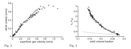
Fig. 3 – Initial settling velocity of the head of the powder bed as a function of the superficial gas velocity to which the powder was previously fluidized.
