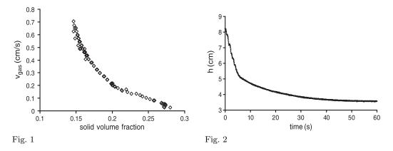
Fig. 1 – Superficial gas velocity as a function of the solid volume fraction of the fluidized powder.
