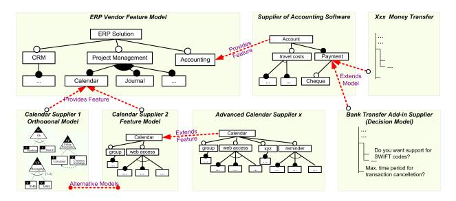
Fig. 1. Example of interrelated multi product lines in the ERP domain. Vendors and suppliers depend on each others' products, hence the variability models are related to each other in different ways. In our approach, the relationships between the models are expressed as IMDI links (see Table II). We have included an OVM model in this example for illustrative purposes only. OVM is not yet supported by the proposed approach.
