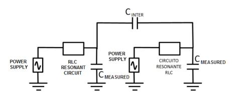
Figure 5. Scheme used in the simulation of interferences between sensor devices.
