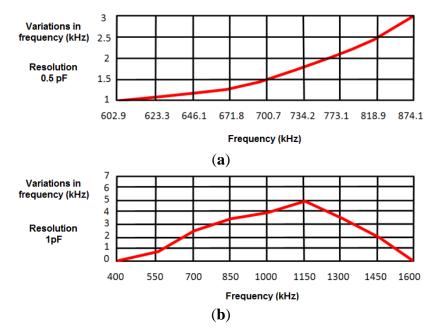
Figure 4b shows the frequency variations produced by a 1 pF increase in human body capacitance. Therefore, the proposed sensor can be considered sensitive to 1 pF variations in the range of frequencies between 508 kHz (50 pF) and 1,488 kHz (200 pF). As shown in Section 4.3, both ranges of sensitivity prove enough to monitor respiratory movements.
