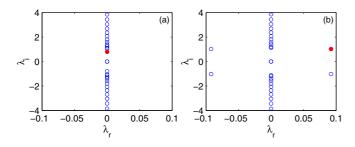
FIG. 6. (Color online) Two case examples of the spectral plane  $(\lambda_r, \lambda_i)$  of eigenvalues  $\lambda = \lambda_r + i\lambda_i$  of the solution for (a)  $b_I = 0$  and (b)  $b_I = 1$ . The eigenvalue which is spectrally stable in the left panel but whose collision with the band edge of the continuous spectrum is responsible for the instability in the right panel is denoted by a red mark.
