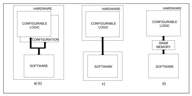
Figure 1. Interfacing models for a Codesign system
