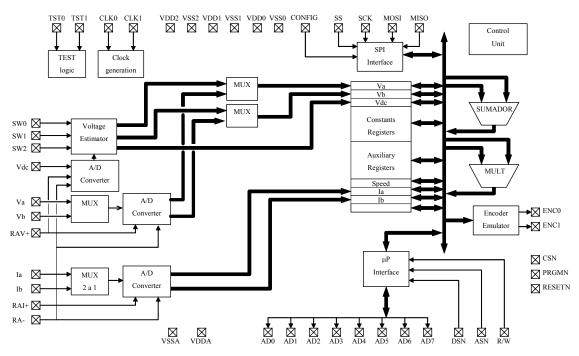
Figure 5. Block Diagram of SLESS ASIC
