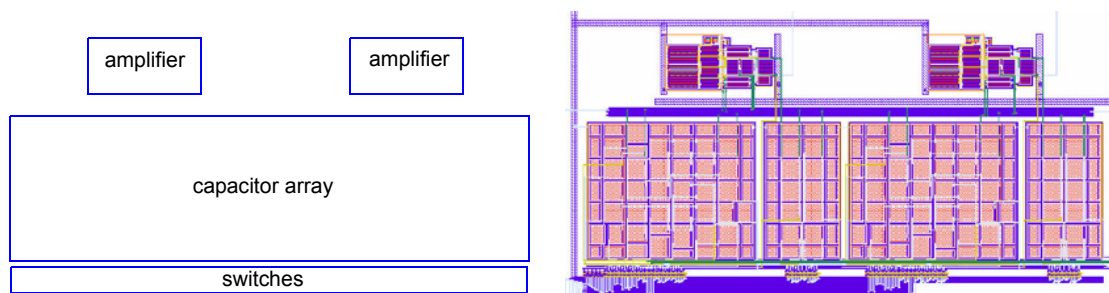
FIGURE 3.26. Floor-planning and layout of the discrete-time SC sinewave generator
