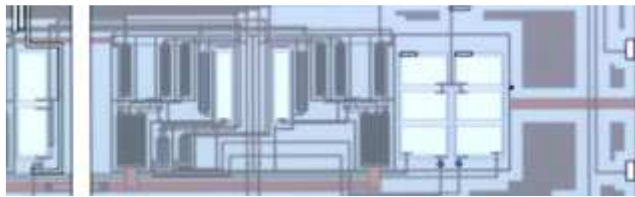
Fig. 5. Micrograph of the class AB transconductor
