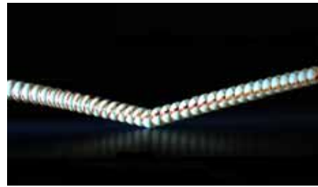
Fig. 3 Overlapped ball images show a spin change from knuckle to top spin at bouncing on the table. The ball flies from right to left.
