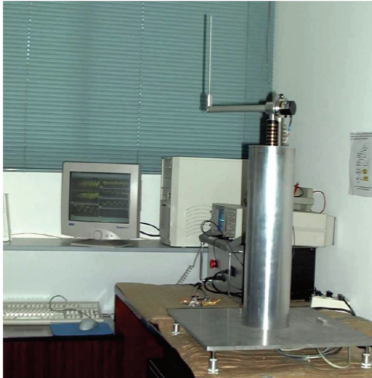
Figure 1: Available Furuta's pendulum.
