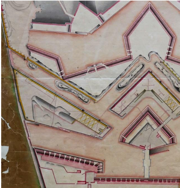
Figure 9. Detail of the plan that shows the state of the Fortifications of the Puerta Tierra of Cadiz, on January 1, 1746. Everything washed in yellow indicates the portion of work done during the year 1745. Municipal Historical Archive of Cadiz.
